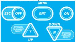
Each button is labelled with its primary function either on the button itself, or adjacent to it. Secondary functions are labelled within a curved white outline next to the relevant button.
