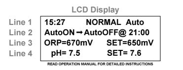
Line 1 shows the current time and the mode of operation. In the example above, line 1, tells you that the time is 3:27pm and the PL Control is operating in "Normal Automatic mode" Note that the PL Control displays the time using a 24 hour clock. Line 2 shows timer information. In the example above, line 2 tells you that the "unit is turned ON and will turn OFF automatically at 21:00 (9pm)"
