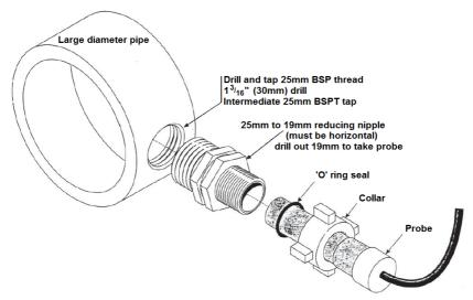
Commercial tap kits are available from pool controls. These include all tools required for a drill and tap installation. (Part number: 08455022)
