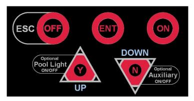
Each button is labelled with its primary function either on the button itself, or adjacent to it. Secondary functions are labelled within a curved white outline next to the relevant button. The buttons are backlit to show which are active at any given time, although the ESC/OFF button is always available to take you back to the home screen.
