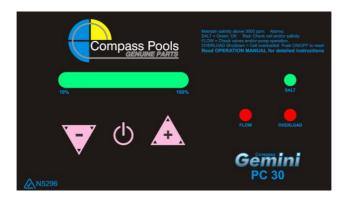
The Gemini Salt Unit uses a simple LED Bar Meter and Alarm LEDs to provide the user with information.
