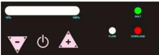
Overload detected, Cell has been turned off.
