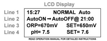
Line 1 shows the current time and the mode of operation. In the example above, line 1, tells you that the time is 3:27pm and the Gemini System is operating in "Normal Automatic mode" Note that the Gemini System displays the time using a 24 hour clock. Line 2 shows timer information.
