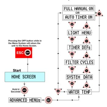
Once you have selected the ADVANCED menu, use the Y/UP and N/DOWN buttons to scroll through the various options. When the name of the sub-menu you require is displayed on the LCD, press ENT to access that sub-menu.
