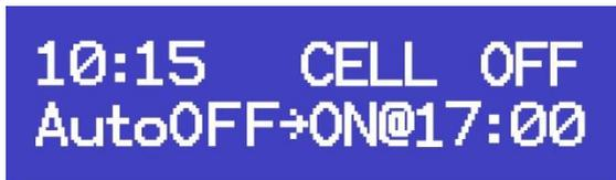
The first line of the display shows the current time and the cell status and output. In the example above the time is 10.15am and the Cell is “OFF”. If the Cell is on, the output of the Cell will be displayed. If the output of the Cell has been set at lower than 100%, “CELL OFF” will be displayed intermittently even while the unit is running as the Cell regulates output. (See Chlorine Output Menu on page 18 for more details)
