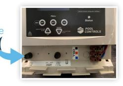
Light Fuse: Unscrew black knob (on right) and lift out. Replace light fuse with a T3.1amp slow burn ceramic fuse
